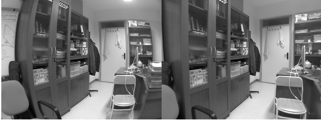
Figure 7: On the left an image which shows radial distortion. On the right the same image after the undistortion.
