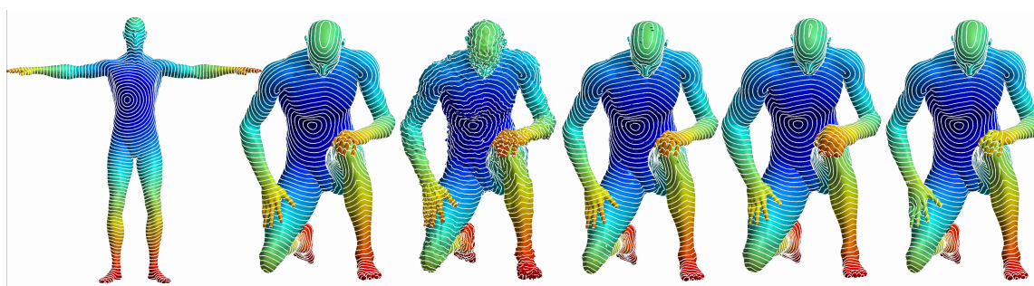
Figure 6.1.: Comparison of the geodesic distance under different deformations of the mesh; from left to right: the null shape, isometry, noise, microholes, local scaling and topology changes.
