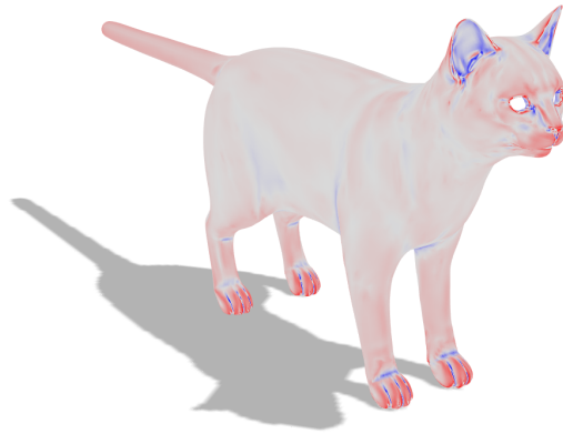
Figure 1.3: Mean curvature of the TOSCA dataset's cat in null-pose on a linear scale from -0.9 (blue) over 0.0 (grey) to 0.9 (red) to highlight extreme values.
