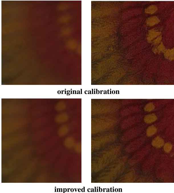
Figure 5. Texture improvements after refining the camera parameters with the proposed approach for the bird data set (see fig. 6). The original calibration was obtained by applying a classical LED-based calibration procedure. Visualized are zoomings of an average texture map (left) and a super-resolution texture map (right). Note the enhancement of the texture pattern as well as the removal of visual artifacts obtained with the refined calibration parameters.
