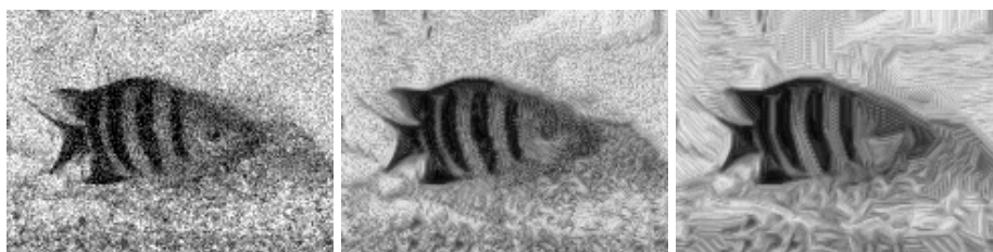
Fig. 6. Hallucination of regular patterns in noise for many iterations and small mask size. From left to right: (a) Gaussian noise with \sigma = 30 added to reference image in Fig.5a. (b,c) Denoising result of the iterated nonlocal means filter with the sorting criterion after 1 and 300 iterations ( n = 10 ). For small n , the iterated filter creates structures from the noise.
