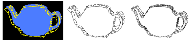
Fig. 4. Left: Projected object surface in blue and the extracted object contour in yellow. One seeks corresponding points between the silhouette of the blue area and the yellow contour. Center: Closest point correspondences. Right: Regularized closest point computed with optical flow numerics and \alpha = 10 .
