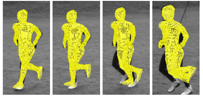
Fig. 18. Illustration of the drift when only flow-based correspondences are used for tracking. From left to right: Result at frames 1, 10, 30, and 150. The optical flow yields good results for the first frames, which indicates its suitability for predicting the pose in successive frames. However, errors accumulate over time and are the reason for tracking failures of the limbs. Successful tracking of the main torso even after 150 frames indicates the generally high precision of the flow-based correspondences.
