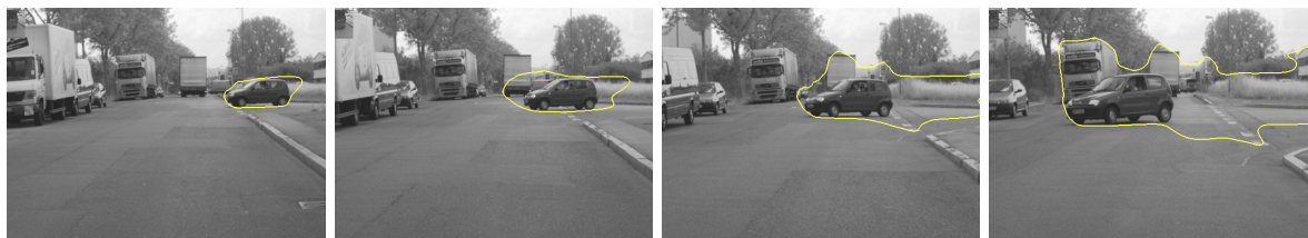
Figure 4: Same setting as in Figure 3 but modeling foreground and background with a global Parzen distribution. Only the strong smoothness constraint ( \nu = 45 ) prevents the contour from capturing even larger parts of the background. Clearly, object and background cannot be distinguished based on spatially uniform feature distributions.
