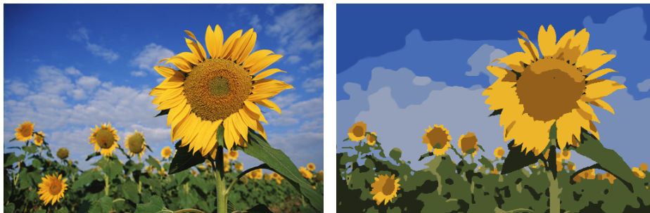
Figure 1: Color input image and segmentation obtained by minimizing the piecewise constant Mumford-Shah functional with 10 regions.
