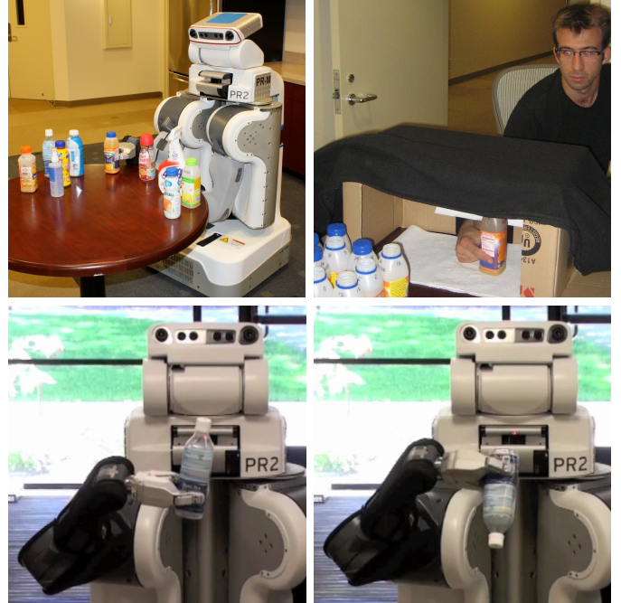
Fig. 1. Top left: A mobile manipulation robot grasping a bottle estimates both object class as well as the state of the grasped object from its tactile appearance. Top right: Comparative study on tactile performance with human test subjects. Bottom: The robot estimates whether liquid is in the bottle by rolling it. The robot extracts peaks of high-frequency using its touch-sensitive fingertips.
