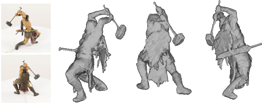
Figure 1.9 Warrior sequence. 2 of 24 input images of resolution 1600 \times 1600 and multiple views of the reconstructed surface. Note that thin structures such as hammer and sword as well as concavities – for example at the chest – are reconstructed accurately.
