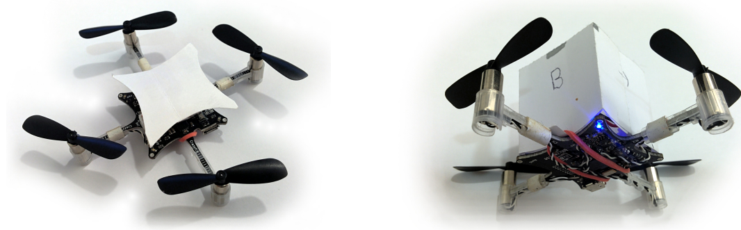
(a) Add paper on the battery to reduce reflections (b) A little paper cube can improve detection distance when using a ceiling mounted Kinect.
