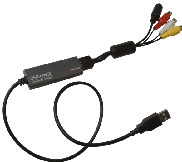
Figure 3.16: The Hauppauge USB-Live2 digitises an analogue video signal (yellow RCA connector) and exposes it to the linux kernel as a video device, much like a webcam.
