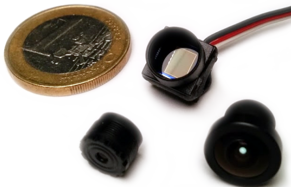
Figure 3.12: The camera and lens used relative to a €1 coin. The small lens on the lower left was shipped with the camera and not used due to its narrow 55^\circ angle field of view. One can see the exposed imaging CMOS of the camera.
