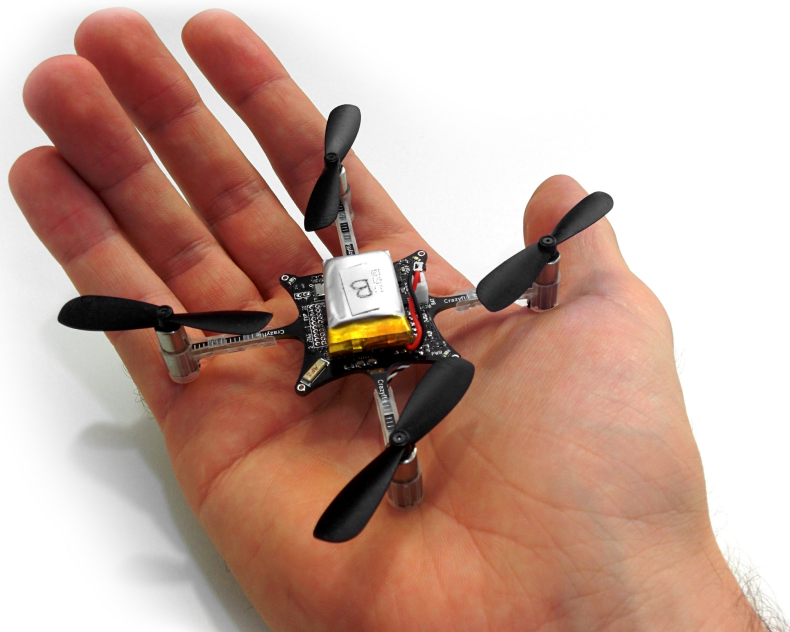
Figure 3.6: At under 19 grams and 8.5 cm across, the Crazyflie can safely take-off from and land on the palm of your hand.
