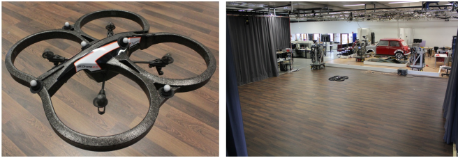
Figure 9: Motion Capture Setup: Left: AR.Drone with attached visual markers; Right: The motion capture volume. The externally tracked pose is solely used for evaluation purposes and at no point to control the quadcopter.
