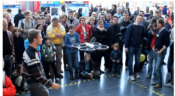
Figure 1: A low-cost quadcopter navigates in unstructured environments using the front camera as its main sensor. The quadcopter is able to hold a position, fly figures with absolute scale, and recover from temporary tracking loss. Picture taken at the TUM open day.
