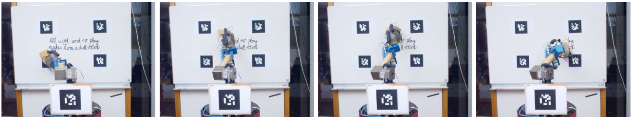
Fig. 8. The reproduction of the board cleaning task by our robot. It imitates the zig-zag movement for cleaning the board with the sponge. Note that the learned task representation allows for cleaning differently sized surfaces based on the markers.
