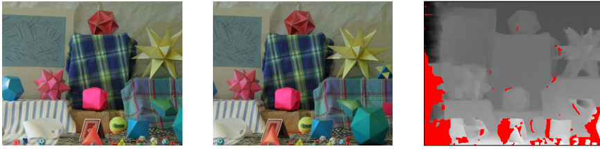
Fig. 9: The proposed method can be employed to simultaneously optimize for a displacement and an occlusion map. This problem is also too large to be solved by alternative relaxation methods on current GPUs. From left to right: Left and right input image I_L and I_R , and computed disparity and occlusion map; red areas denote occluded pixels.
