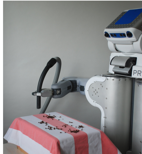
Fig. 1: Experimental setup. The PR2 cleans a table with a vacuum cleaner. Instead of cleaning the whole table, the robot observes the outcome of its actions, learns which features correspond to dirt, and cleans these regions.
