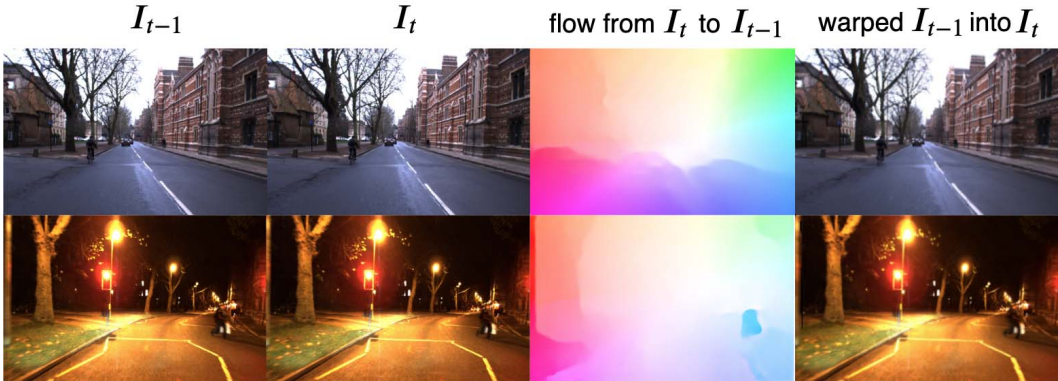
Figure 4: Flow estimation and warped images of Day and Night scene in the Oxford RobotCar dataset. The first row is made of images of Day set and the second row consists of images from Night set. The estimated flows show the fair quality of warped images leading to reasonable supervision for consistency.
