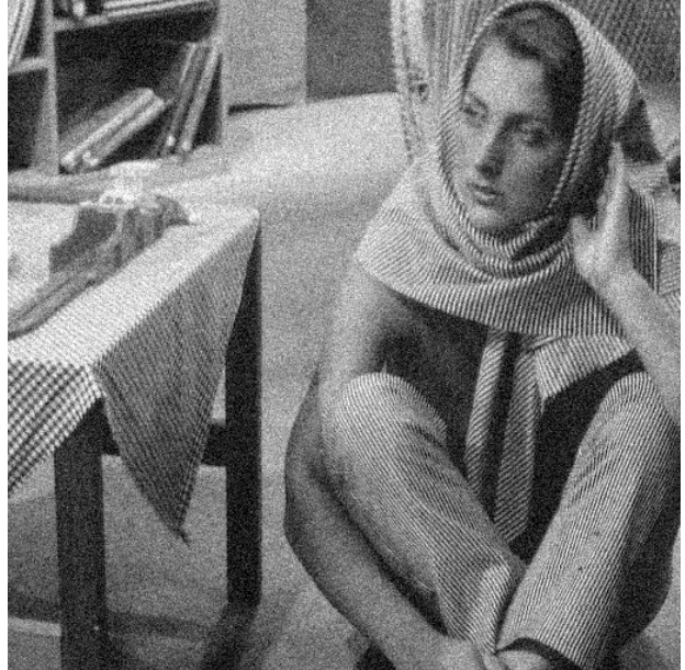
Figure 4. Standard test image Barbara of size 512 \times 512 pixels including Gaussian noise with standard deviation 20 as used in the experiments.
