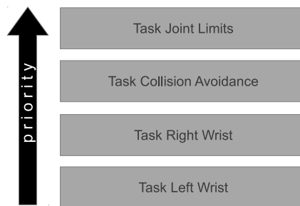
Figure 6.2.: Basic hierarchy stack of used tasks for the experiments. As illustrated, joint limits have always the highest priority. The collision avoidance task takes precedence over the tasks of interest such as the right or left wrist. In the conducted experiments, we will also examine the behavior of changing the order of left and right, yet constantly placing them at least priority.
