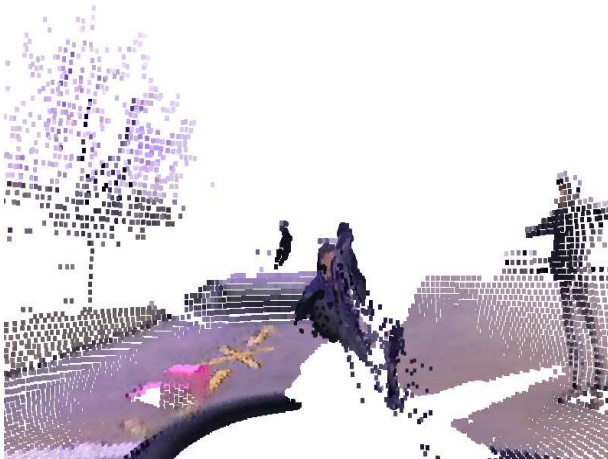
Fig. 7. 3D scan with texture. One recognize a tree on the left hand side, yellow street markings (-x- shape), a pink box (next to the street markings) and persons (e.g. on the right, with arms extended)
