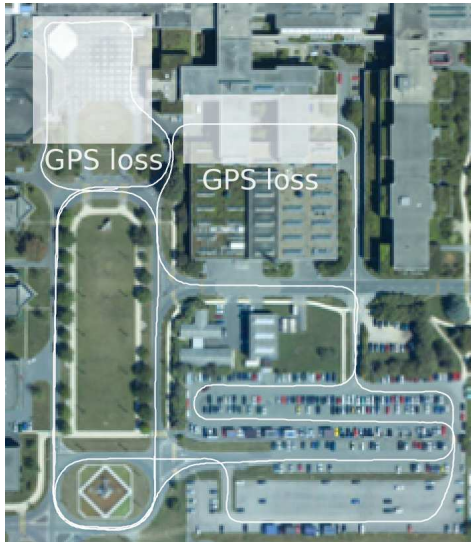
Fig. 11. Overlay of the estimated trajectory on the ortho-photo of EPFL. The areas where the GPS was not available are highlighted. The total travelled distance was 2350m.
