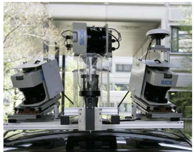
Fig. 4. Sensors mounted on the roof
