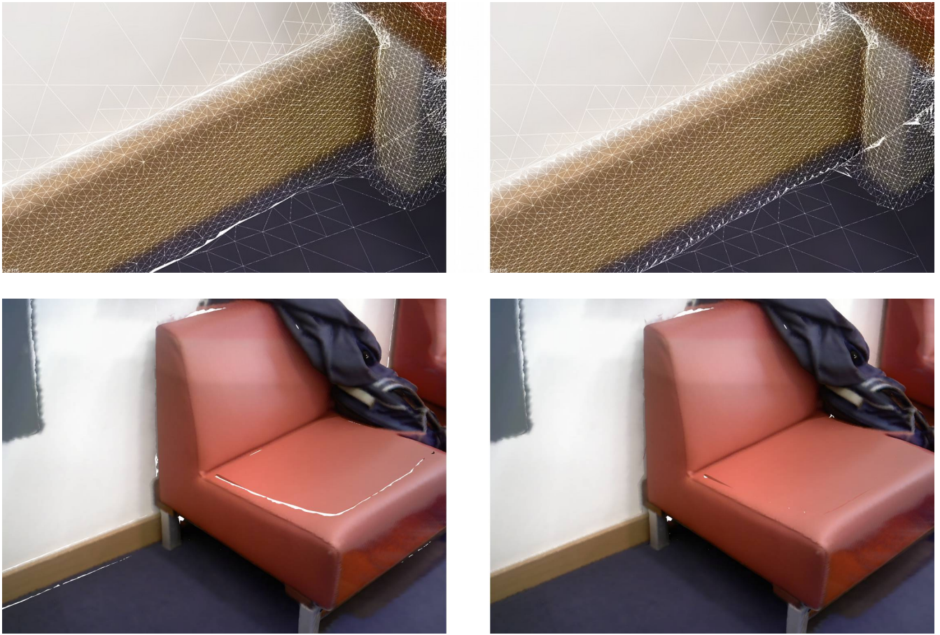
Fig. 9: Joining of GPT mesh with planar segment triangulations. Left shows unjoined segments and right shows segments joined with interpolated boundary vertices.
