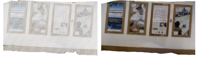
Fig. 6: Texture generation, from left to right: (a) plane segment from a colored point cloud; (b) generated texture.
