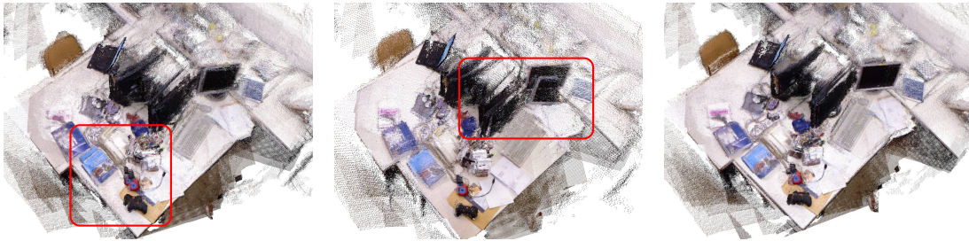
Fig. 5: Comparison of accumulated point clouds from keyframes using SLAM. From left to right: tracking without planes, hard labeling the planes, and soft labeling the planes (our EM approach).
