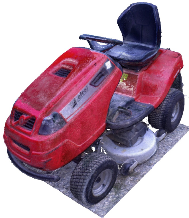
Figure 1.2: The 3D model of a lawn tractor, which was reconstructed using the approach developed in this thesis. Such workpiece reconstructions allow visual inspections as well as metric measurements.
