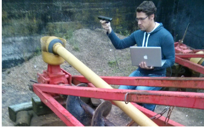
Figure 4.3: RGB-D data of a workpiece is acquired by using a hand-held RGB-D sensor at a distance roughly between 0.70 m and 1.80 m to the surface.
