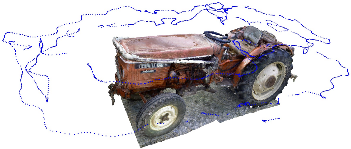
Figure 5.17: Reconstructed 3D model of the WR/tractor dataset together with the corresponding estimated camera trajectory.
