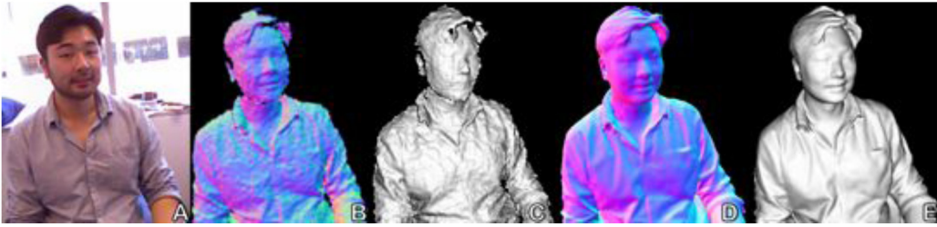
Figure 2.2: RGB image (A), surface normals (B) and noisy surface reconstruction (C) from a single bilateral filtered input frame. (D) and (E) show the surface normals and the Phong shaded model of a 3D model generated from KinectFusion. [24].
