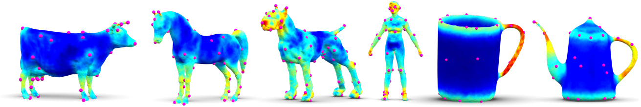
Figure 4. Saliency maps computed with AWFT on some shapes from the evaluation benchmark. The areas considered as more salient are in red while the less important ones tend to blue. The final selected points are highlighted by small pink spheres.
