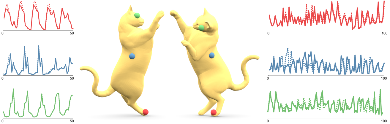
Figure 6. Comparison between WFT (left) and AWFT (right) descriptor computed at three symmetric points of the cat shape (points and corresponding curves are color-coded). Solid and dotted curves represent descriptors from the left and right side of the cat, respectively.
