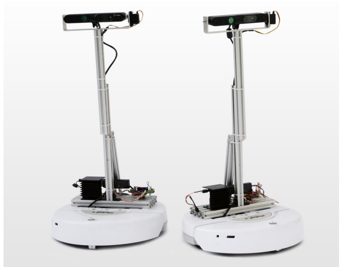
Fig. 3: The two low-cost ( < 600\$ ) robots used in our evaluations: Each robot consists mainly of a differential drive base (iRobot Create), an RGB-D sensor (PrimeSense), an ARM-based single board computer (ODROID-U2), and a dual band USB wireless device.
