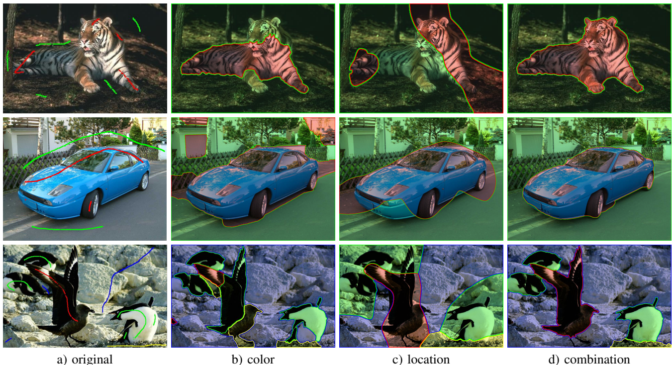
Fig. 2. a) Original images with strong lighting variations and reflections. b) Segmentation results based on color similarity only. c) Segmentation results based on scribble distance only (i.e. a length-regularized Voronoi tessellation). d) Segmentation results based on spatial and color information of the scribbles.
