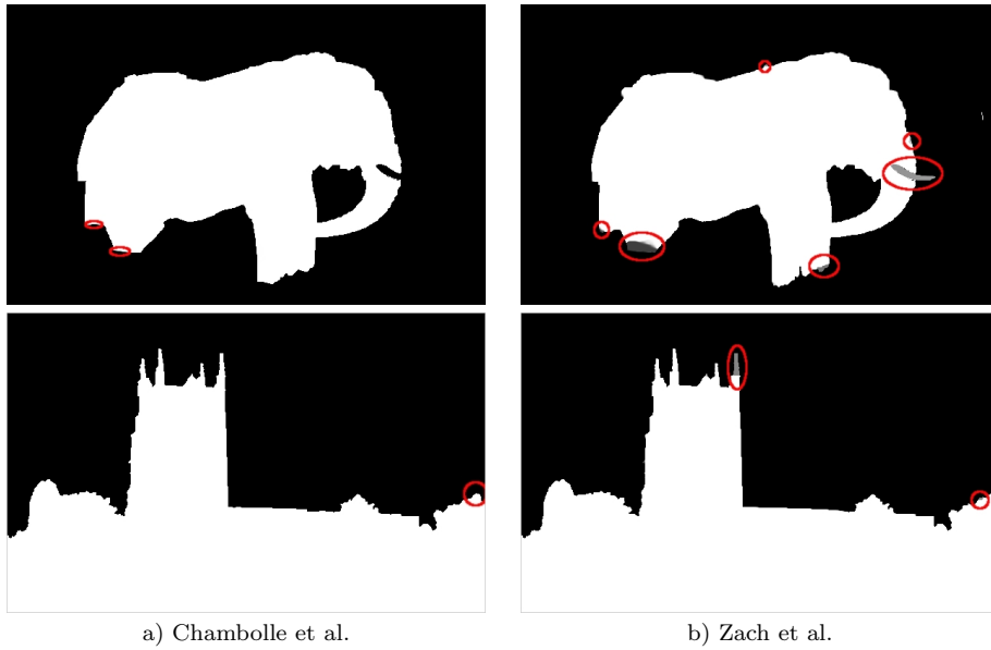
Fig. 6 Results of the relaxed optimization problems before binarization a) by Chambolle et al. and b) by Zach et al. The fact that the indicator functions are non-binary in very few locations only (marked by red circles) indicates near-optimality of the computed solutions.
