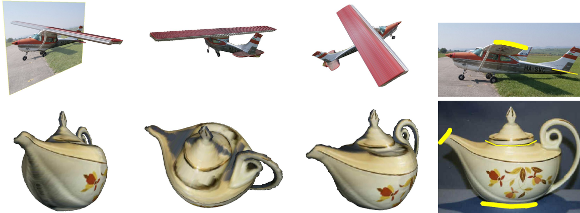
Figure 7. Reconstruction results with user input altering the local smoothness of the surface. Next to the reconstructions the input images are shown with the respective user scribbles. User scribbles (yellow) decrease the surface smoothness locally.
