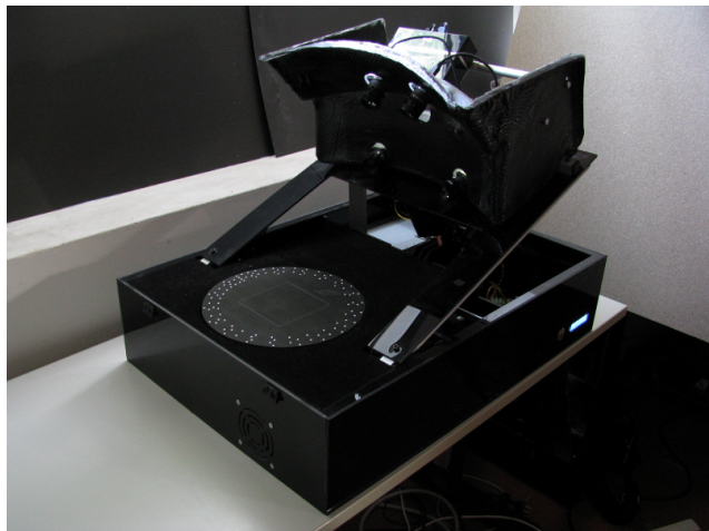
Figure 3. The general purpose structured light scanner used.
