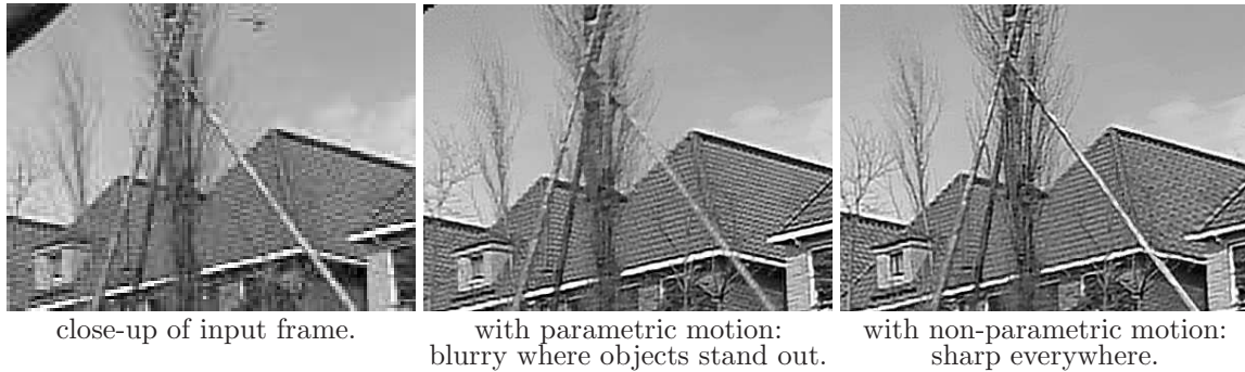
Figure 5.12.: Non-parametric motion models are needed when there are objects with different depths in the same layer.
