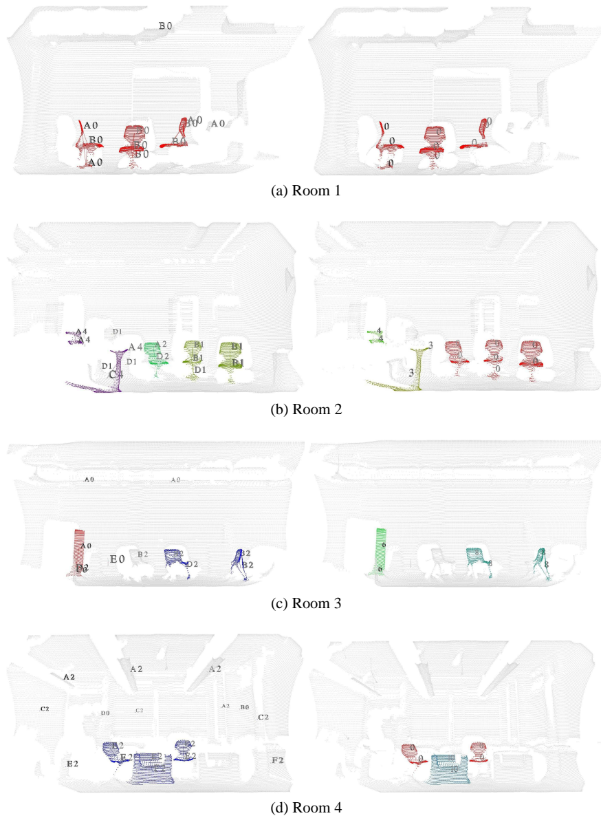
Fig. 10: Results of category discovery. Left images contain objects discovered through the object discovery process, and right images are the same objects after categorization. Objects in the left images are colored according to their local class labels while objects in the right images are colored by their global category labels. Notice that the categorization step can correct incorrect classifications of the discovery step.
