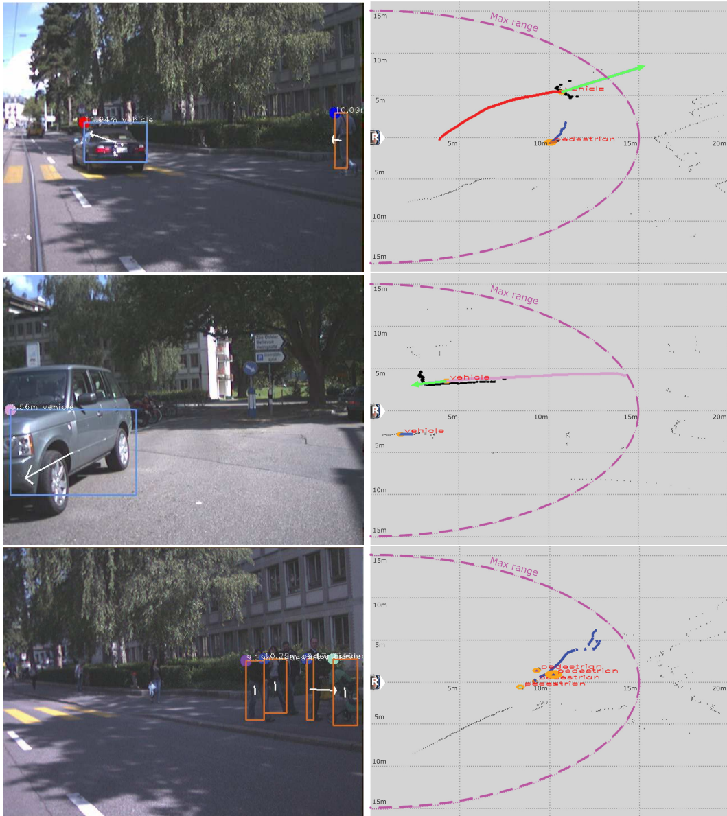
Figure 12: Cars and pedestrian detected and tracked under occlusion, clutter and partial views. In the camera images, left column, blue boxes indicate car detections, orange boxes pedestrian detections. The colored circle on the upper left corner of each box is the track identifier. Tracks are shown in color in the right column and plotted with respect to the robot reference frame. Green vectors show direction of motion for cars.
