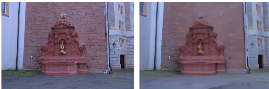
Fig. 8. Left: One real view of the object 'fountain-P11' [13]. Right: Colored estimated albedo, using the proposed approach. Geometry and camera parameters estimates are outputs of an SfM/MVS pipeline using 25 input images. Only 8 images have been used as inputs of our algorithm.
