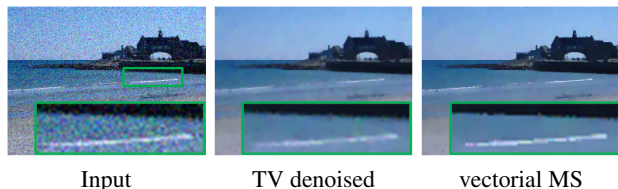
Figure 1. We propose a convex relaxation and an efficient implementation for the vectorial Mumford-Shah functional. It allows to compute piecewise smooth approximations of color images independent of initialization. Compared to the Total Variation ( center ), the Mumford-Shah model ( right ) preserves image contrast.
