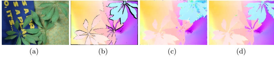
Fig. 1. (a) input image 0 of the Middlebury “Schefflera” sequence; (b) color-coded ground truth flow (hue = direction, intensity = magnitude, black = unknown); color-coded flows, estimated using: (c) a continuous TV- L^1 flow model; (d) the proposed optimization strategy (AAE = 2.91°)
