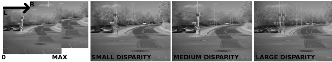
Fig. 8. Idea of plane sweep stereo . The right image is translated according to a given disparity value, and the consistency of gray values in the left image and the translated right image corresponds to the likelihood of a stereo match. The superposition of the right and left images for different disparity values results in sharp structures in the background (for small disparities), midplane, or foreground (for large disparities).
