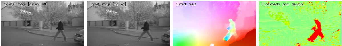
Figure 3: Optical flow for a scene with a running person and a moving camera, installed in a vehicle. Flow above 15px is color-saturated. The distance to the epipolar rays encodes independently moving objects. Clearly, the running person becomes visible ( \lambda_{1,2} as in figure 2).
