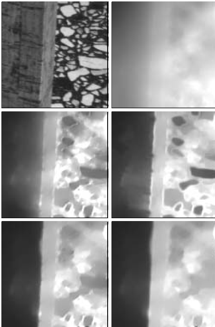
Figure 3: (a) TOP LEFT: Detail from the lower right part of Frame 16 ( 128 \times 128 pixels). (b) TOP RIGHT: Optic flow magnitude for homogeneous regularization. (c) MIDDLE LEFT: Image-driven isotropic regularization (d) MIDDLE RIGHT: Image-driven anisotropic regularization. (e) BOTTOM LEFT: Flow-driven isotropic regularization (f) BOTTOM RIGHT: Flow-driven anisotropic regularization. For better visibility, the grey values of the optic flow results been transformed by a gamma correction with \gamma = 0.4 . From [36].
